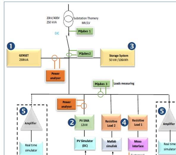
Figure 1 – Overview of the microgrid used infrastructure
