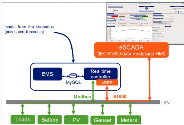
Figure 2 - Microgrid infrastructure for the grid-connected mode
