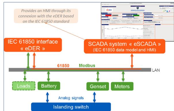
Figure 3 – Microgrid infrastructure for the islanding mode
