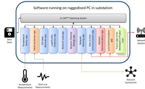
Figure 2: LV-CAP™ OS & software applications
