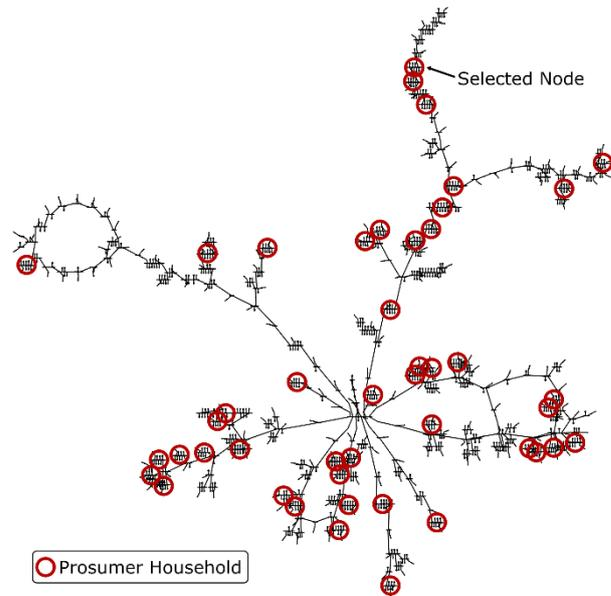
Figure 1 Topology of the simulated low-voltage grid
