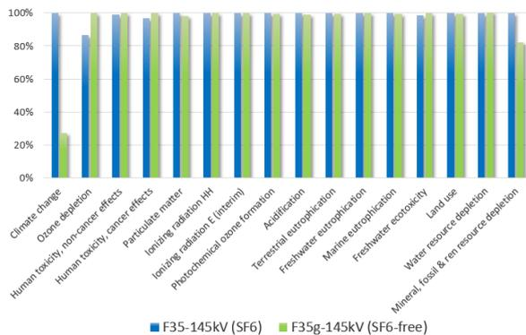
Fig. 9: LCA comparison of F35-145kV (SF<sub>6</sub>) in blue and F35g-145kV (SF<sub>6</sub>-free) in green.
