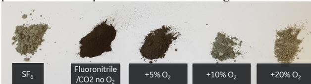
Fig. 2: Powders formed in  $g^3$  with different oxygen content, compared to  $SF_6$ .
