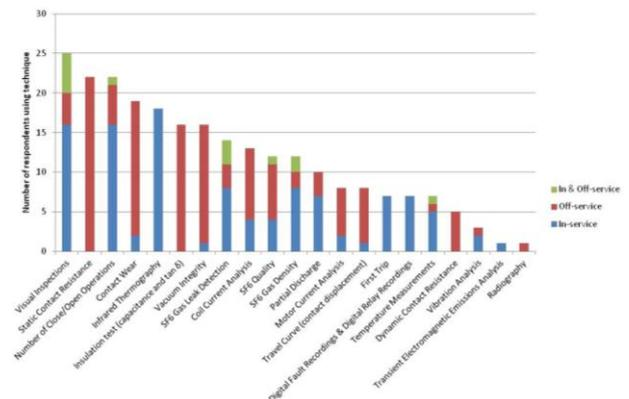
**Figure 2:** List of switchgear non-intrusive condition methods, identified through the international utility survey.
