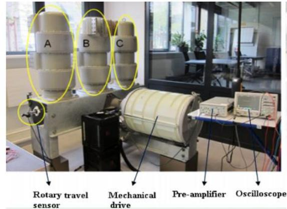
**Figure 5:** Measuring setup for 3 pole circuit breakers [7]
