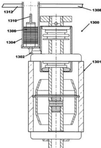
**Figure 4:** Pressure monitoring via an additional bellows (1306) attached to the VI. A tube connects the additional bellows to the VI (1302), and the movement of part (1310) during loss of vacuum breaks the light path between (1308) and (1312) [5].
