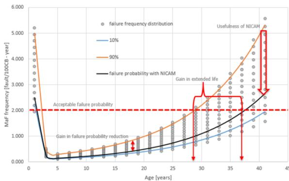
**Figure 1:** Principle representation of frequency of major failure and failure probability curves as a function of the age of asset
