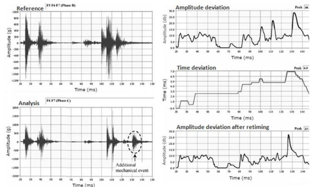
**Figure 6:** Graphs of the vibration analysis on a circuit breaker
