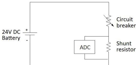
Fig. 1: Circuit diagram for measuring current using the new tool.
