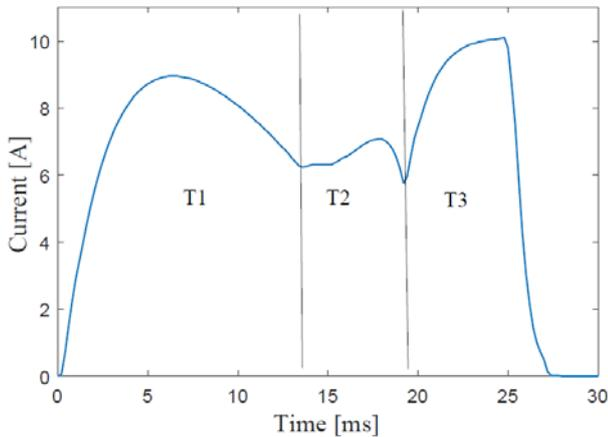
Fig.4 Trip current pattern under normal operation of CB.
