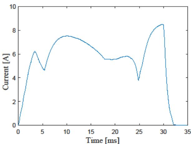
Fig.6 Trip current waveform during relay contact problem. The current rise during the time period T1 is not linear as compared to Fig. 4.
