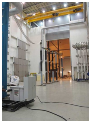
Fig. 5: Superimposed impulse testing of HVDC cable.
