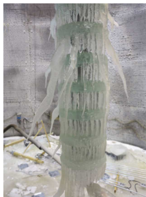
Fig. 2: Ice test on glass cap & pin insulators.
