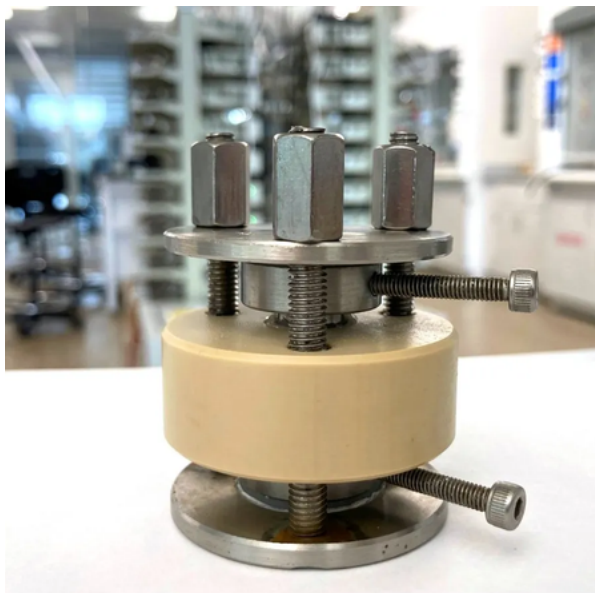
This prototype anode-free all-solid-state lithium battery can store twice as much energy as conventional, liquid-electrolyte or gel-based-electrolyte lithium-ion cells. YIXIAN WANG/UNIVERSITY OF TEXAS AT AUSTIN
