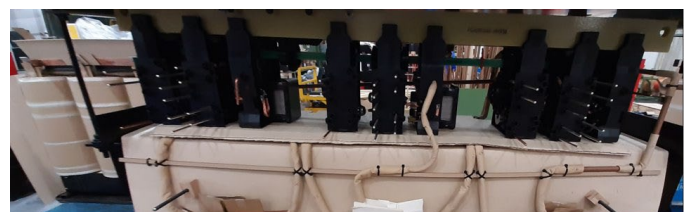
Fig. 3 Tap Changer in low loss 1 MVA Transformer.
