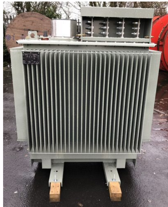
Fig. 3 630kVA Ester Transformer with peak capability > 900kVA
