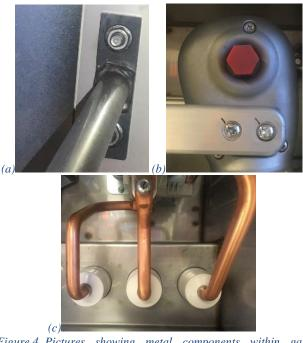
Figure 4. Pictures showing metal components within gas enclosure of field test unit after 3 years of service. (a) Stainless steel internal supporting rod welded to stainless steel plate, (b) cast aluminum vacuum interrupter pole house and extruded aluminum bus bar and (c) bare copper conductors.
