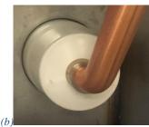
Figure 5. Pictures showing polymer parts from returned and opened field test switchgear. (a) Molded glass fiber filled PBT parts and (b) cast epoxy bushing.
