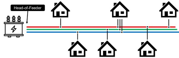
Figure 1. Illustration of a three-phase LV feeder.
