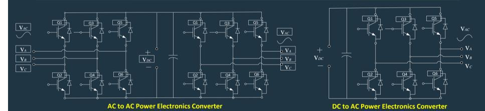
PECs use high-frequency switching devices such as IGBTs and MOSFETs to convert a DC or AC voltage to a voltage with waveform, frequency, phase and amplitude required by the load or utility grid.
