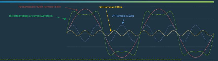
In an ideal world, voltage and current waveforms are perfectly sinusoidal. In the real world, however, they are often distorted by nonlinear loads or sources.
