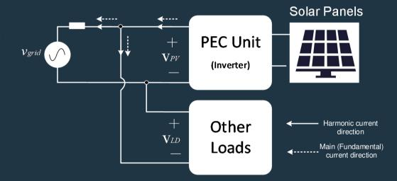
The output current from PEC unit has fundamental 50Hz and harmonics components.
