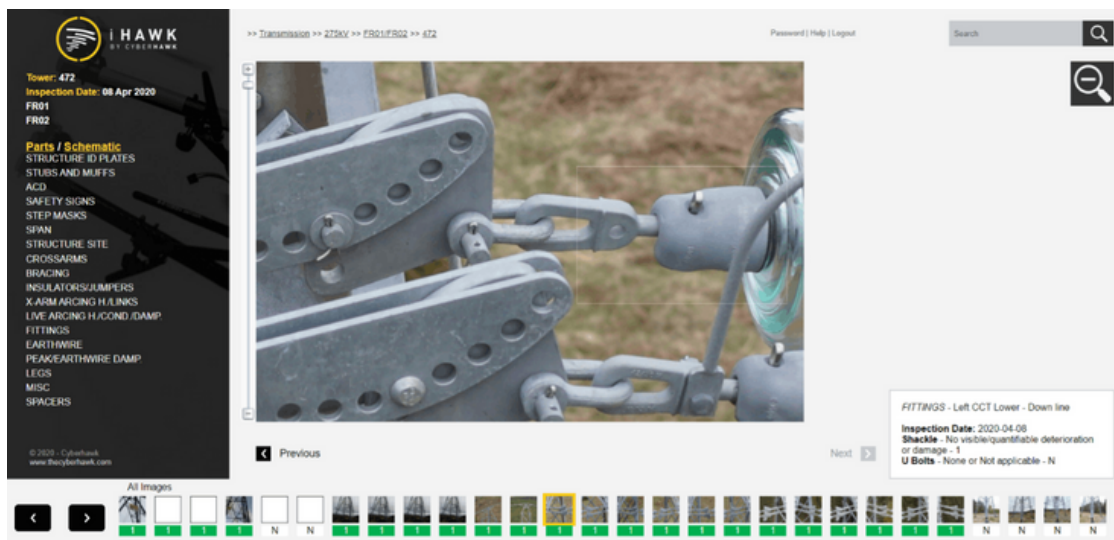
Insulator fitting with missing split pin.
