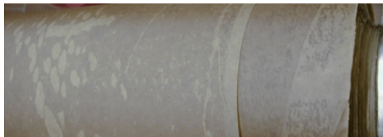
Oil-impregnated paper insulation.
