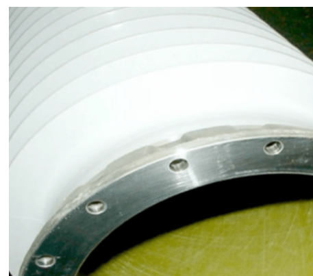
Composite insulator with hydrophobic silicone sheds.
