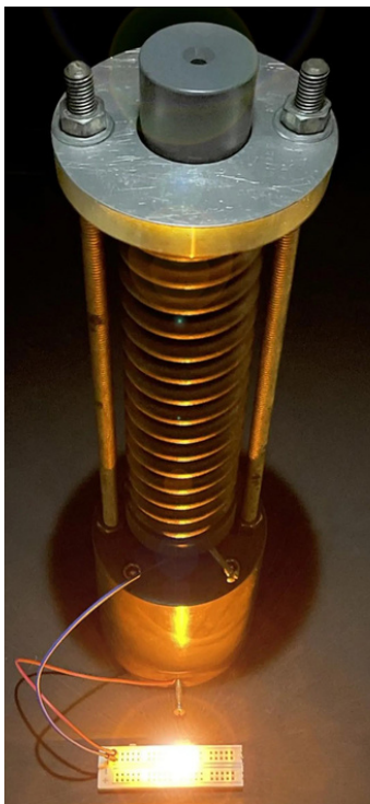
This new supercapacitor can be easily scaled thanks to its large internal surface area of conductive material created by using carbon black. FRANZ-JOSEF ULM, ADMIR MASIC, AND YANG-SHAO HORN/MIT
