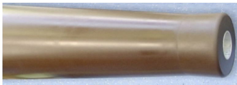
Resin-impregnated paper insulation.
