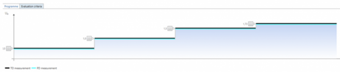
Fig. 2: Sequence of parallel VLF TD and VLF PD diagnostics.
