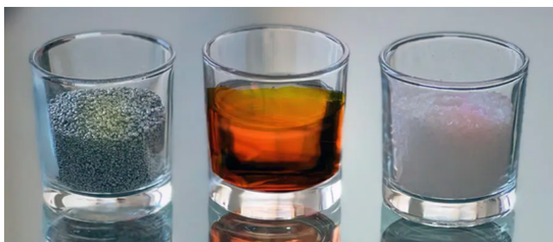
The three primary constituents of the battery are aluminum (left), sulfur (center), and rock salt crystals (right). Image: Rebecca Miller
